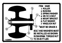
Type A Anti-Scalp Rollers – See Figure 12 PART NO. 1-323540
